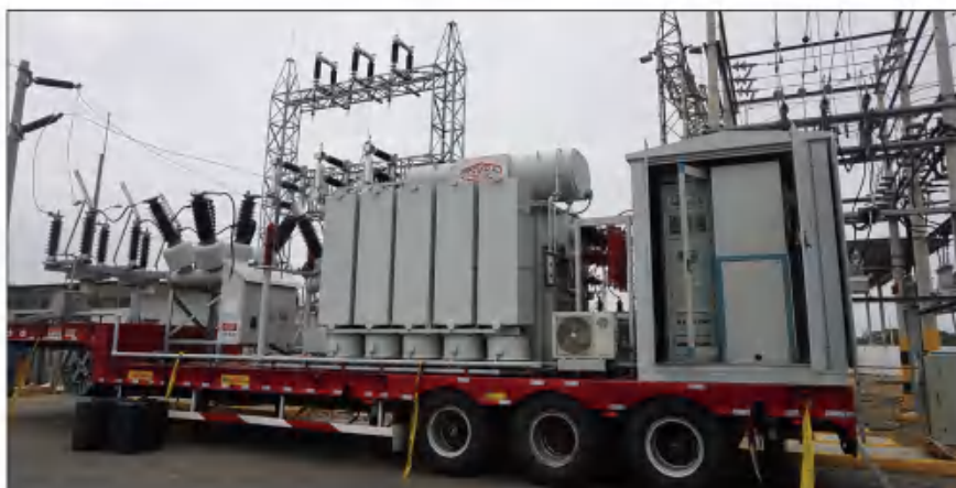
69KV Mobile Substation operating in Ecuador
