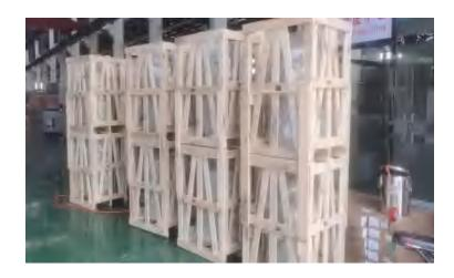
For single phase transformer, we used the wooden frame structure for the capacity up to 50kva, so it will save space and sea shipping cost.
